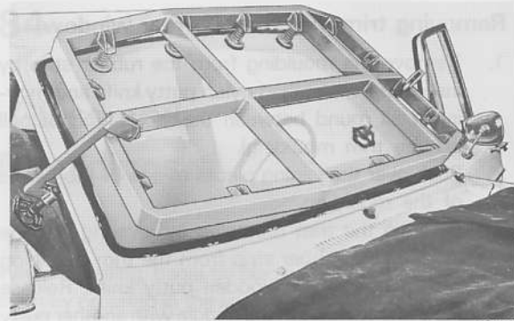
Using fixture 2899 to install windshield
