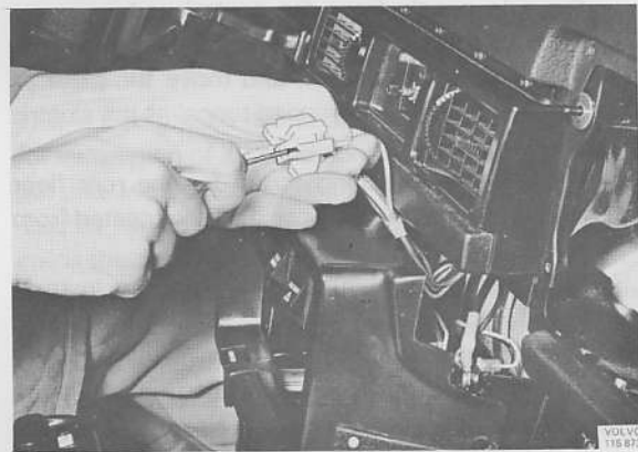
Removing electric cables for contact unit
