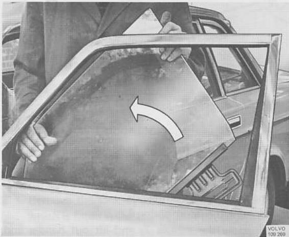
Door window removal
