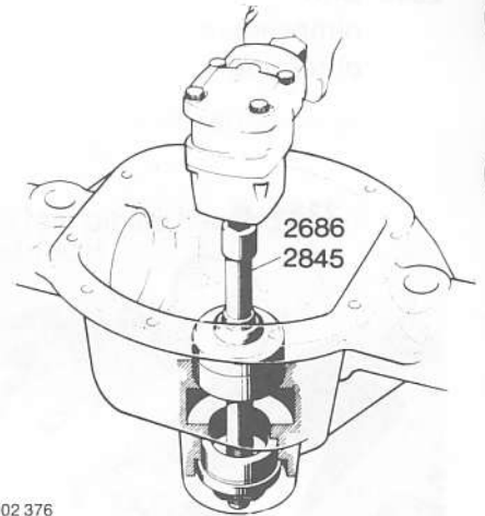
102 376 2686 Press tool installing pinion bearing outer rings 2845 Press tool installing pinion bearing outer rings
