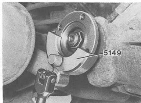
128 808 5149 Wrench installing/removing drive flange
